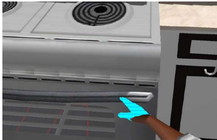
Figure 8. Wall Vision Effect Showing that the Avatar's Hand Has Overreached into a Virtual Object
